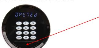
Initially the keypad may not have batteries fitted. To insert batteries pull the door open, remove the grey cover from inside the drawer and load 4pcs 1.5V AA Alkaline batteries. Replace the battery cover.
